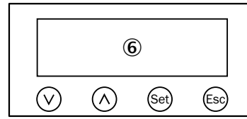
⑥ Liquid crystal display with funktion keys
