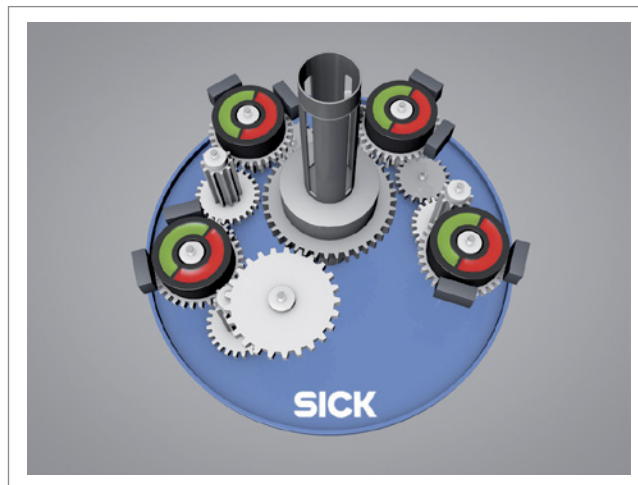
Example: Magnetic multiturn with gearing.
