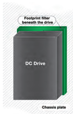
Drive mounted on an external footprint filter
